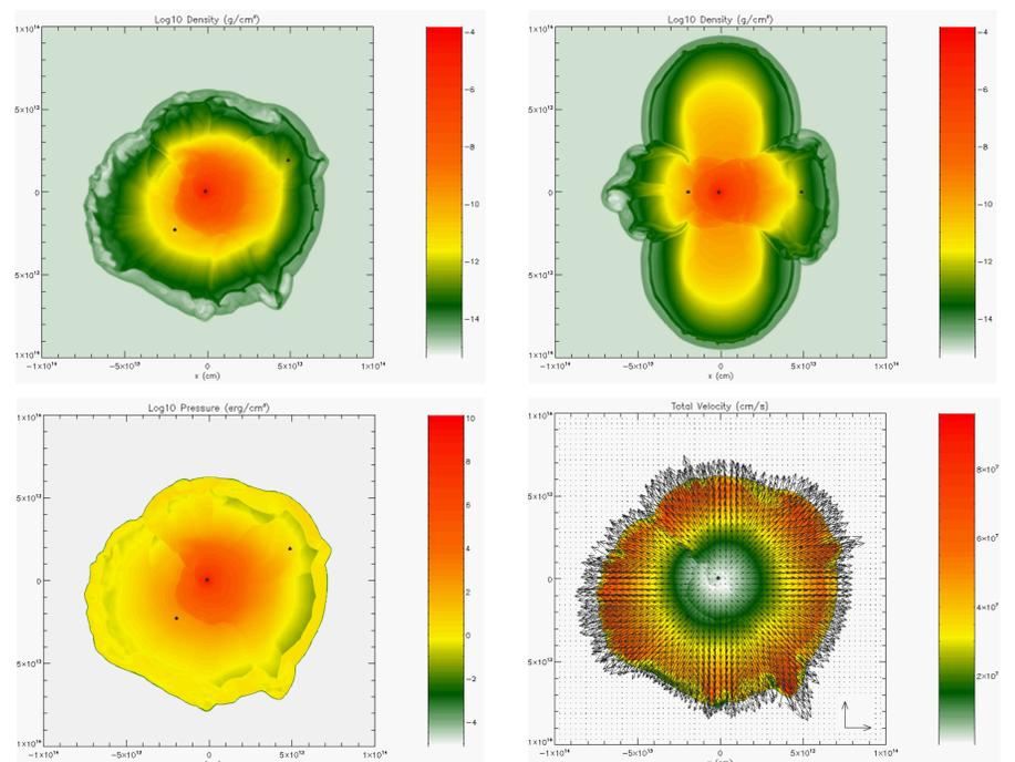
**Figure 3:** Top left to bottom right shows (a) density in the x,y-plane, (b) density in the x,z-plane, (c) pressure in the x,y-plane and (d) total velocity overplotted with velocity vectors scaled to 60km/s in the x,y-plane. All images show the evolution after 0.27 years.
