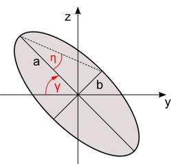
$$\begin{aligned} I &= C_{\text{abs}} \cdot B_{\lambda}(T) \\ Q &= I \cdot \cos 2\eta \cos 2\gamma \\ U &= I \cdot \cos 2\eta \sin 2\gamma \\ V &= I \cdot \sin 2\eta \\ |\tan \eta| &= b/a = \sin \theta_{\text{obs}} \cdot \cos \varphi_{\text{obs}} \end{aligned}$$
