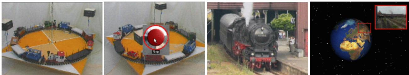
A tele-experiment has been set up, where a toy train circles on a support, with a central suspension. Controlled by an applet and observed by a WEB-cam the law of conservation of angular momentum could be demonstrated.
